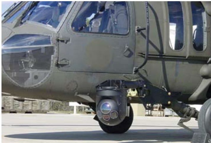
Sponson Sensor Mount with FLIR sensor
